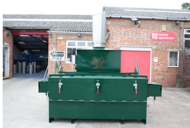
Volkan 750 incinerator suitable for small abattoir use 58
